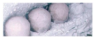
Chartek® Bolt Caps retain material integrity both during and after the effects of fire. Therefore protecting the underlying bolt connections against embrittlement, a result of rapid quenching from firefighters, hose stream.
